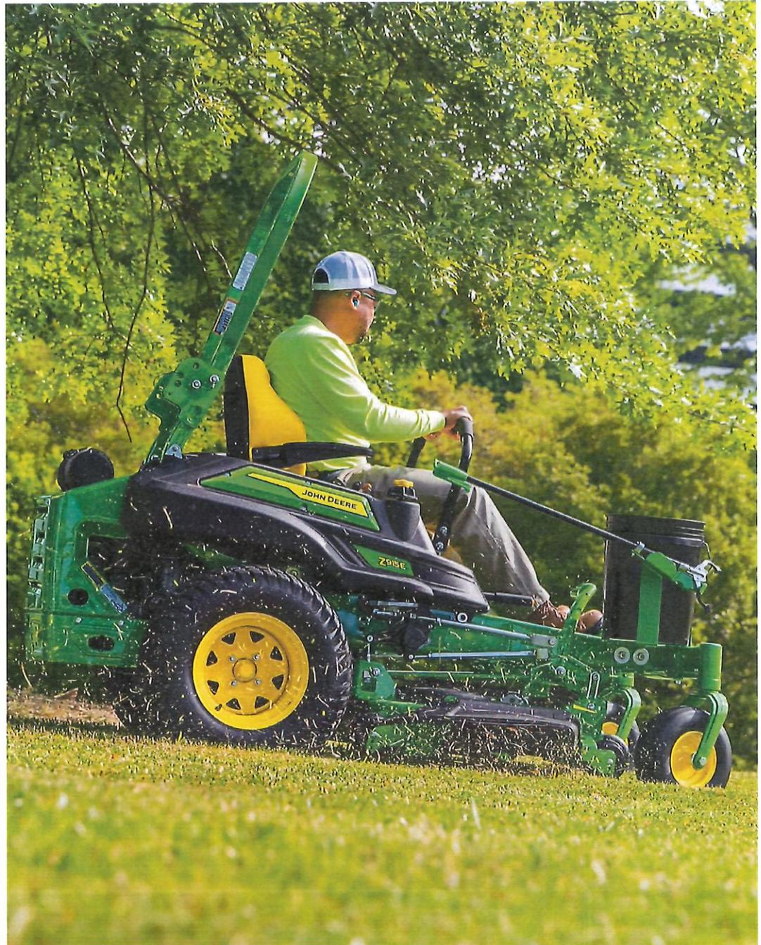
Foldable Rollover Protective Structure (ROPS) and retractable seat belt are standard equipment on Z900 ZTrak mowers.
