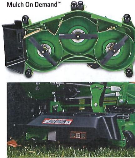
Lastly, if you need to mow right to the edge, there's the FastBack™ PRO Rear Discharge deck. A unique baffling system reduces clumping and windrowing often associated with rear-discharge decks. So less clippings get on the operator and stay where they should: in the turf.
