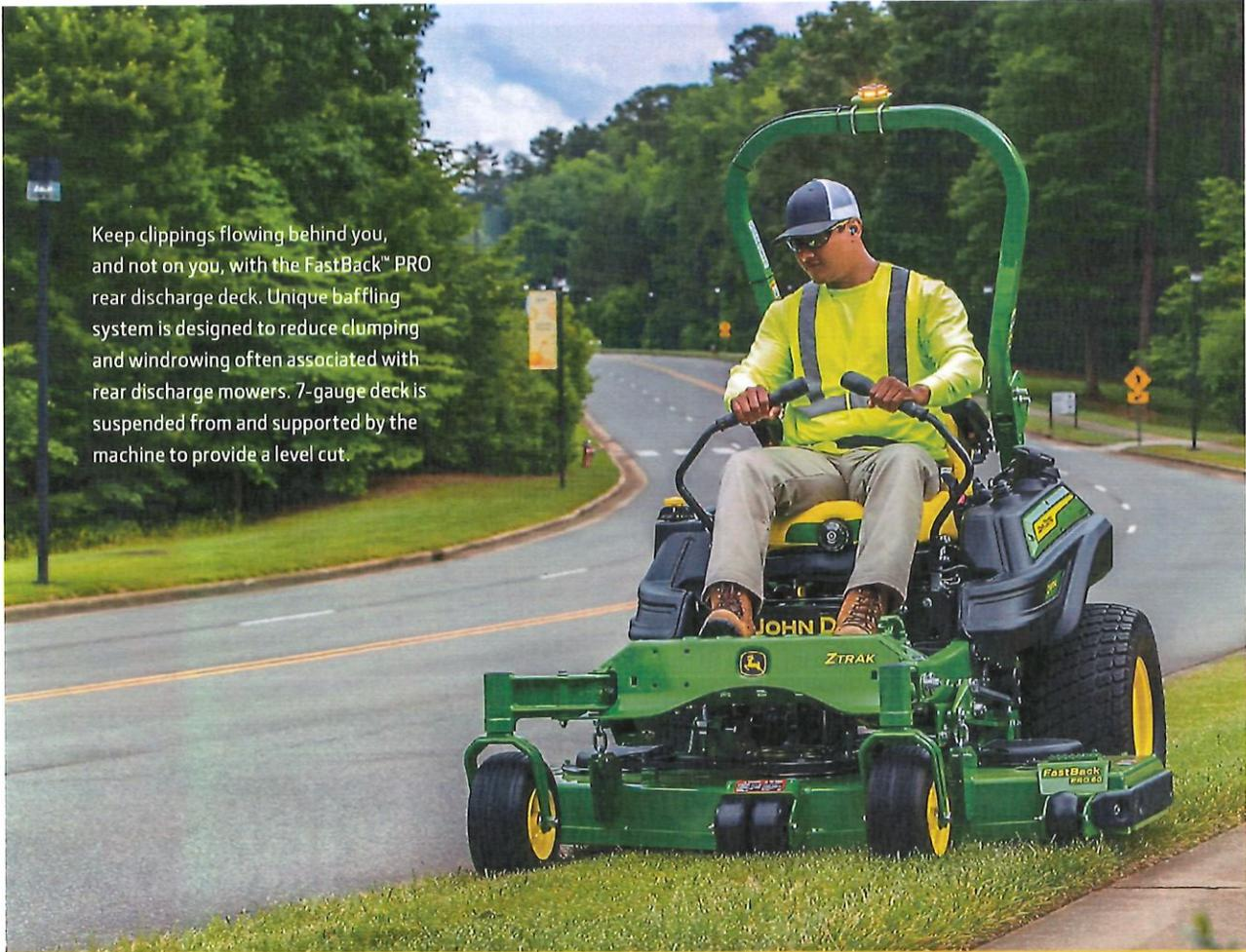
Keep clippings flowing behind you, and not on you, with the FastBack™ PRO rear discharge deck. Unique baffling system is designed to reduce clumping and windrowing often associated with rear discharge mowers. 7-gauge deck is suspended from and supported by the machine to provide a level cut.
