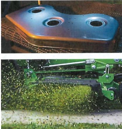
And when it comes to a mulching deck, nothing can touch our Mulch On Demand™ deck. Because we put the power to choose mulching or side-discharge at your fingertips. By shifting the lever to mulch position, the movable gate closes off the discharge chute.
